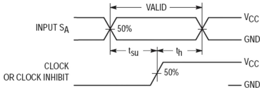
Figure 5. Serial-Shift Mode
