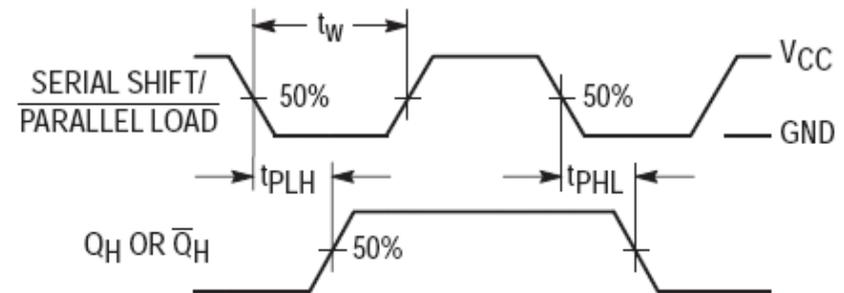
Figure 2. Parallel-Load Mode
