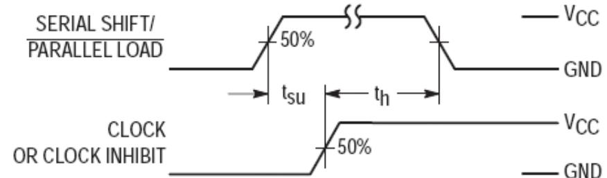
Figure 6. Serial-Shift Mode
