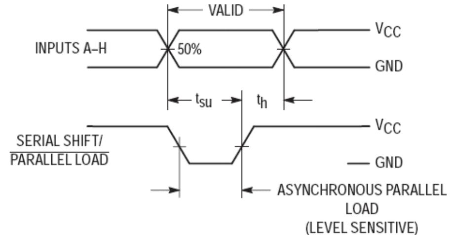
Figure 4. Parallel-Load Mode
