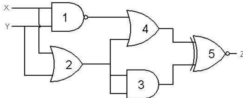
$$\overline{\underbrace{(\underbrace{X \cdot Y}_1) + (\underbrace{X + Y}_2)}_4} \oplus \underbrace{(\underbrace{X + Y}_2) \cdot (\underbrace{X + Y}_2)}_3} = Z$$
